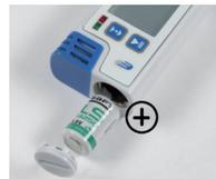
Remove empty battery and insert new battery like shown.
