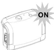
The low pressure indicator (yellow LED) will illuminate while the mattress is pressurizing.
